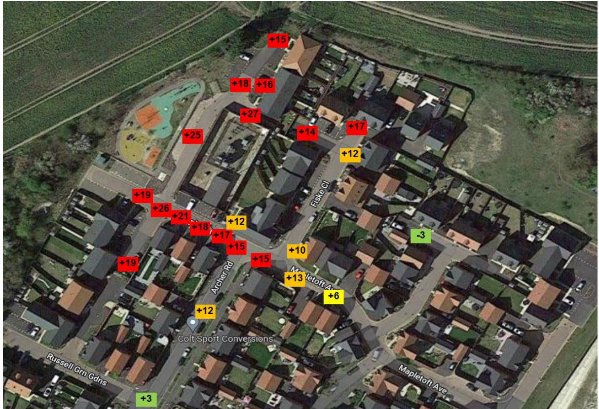
Figure 7.1 – Difference between rating level and background sound level (BS4142), based on measured noise levels 11-12 th October 2022.
